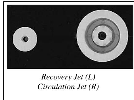
The Recovery Jet is a small jet above the spa water level. It may look the same as the small Circulation Jet, or it could be a round cap, about an inch in diameter. This jet is designed to draw air from the space between your spa water and the spa cover. If your spa is equipped with an Ozone Generator, this air is charged with the cleansing agent (a gas)
