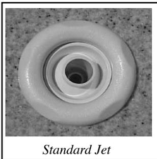
You can adjust both the direction and the velocity of water flow from the Standard Jets. The water flow can be reduced by turning the center nozzle or outer ring (depending on the model) clockwise. By closing one jet, the pressure in the other jets is increased.
